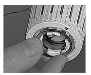
**3)** Insert the toothed ring in the head in such a way that the projecting tooth corresponds to the appropriate slot on the inside of the knob. When these steps have been completed, replace the cover, making sure it locks into position.
