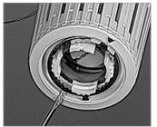
**2)** Remove the metal toothed ring from its seat by extracting it from the thermostatic head with the help of the screwdriver. During these operations, do not turn the knob on the thermostatic head or the calibration position will be lost.
