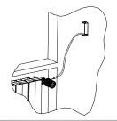
**6)** Install the adjustment knob at the desired distance, using the installation kit included with the package.
